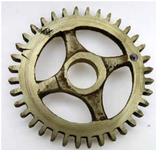
Figure 11. The hour wheel with alignment marks (left). An iron pin filed flush indicates its former use as a reverse minute-wheel, possibly from a small turret clock. The crossings are of an unusual section for a clock.
