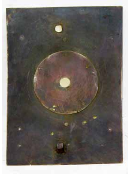
Fig. 14. Rear of the dial with the insertion of a thicker central section.
