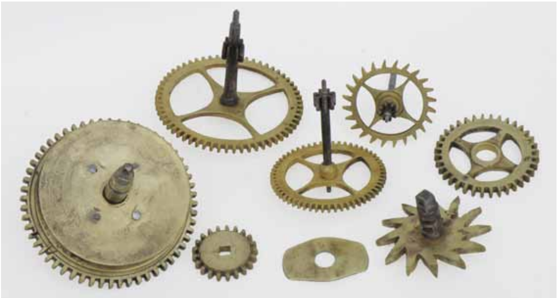
Fig. 10. The four wheels of the going train after conversion to long pendulum and anchor escapement, together with the starwheel and later pinion of report and hour wheel.
