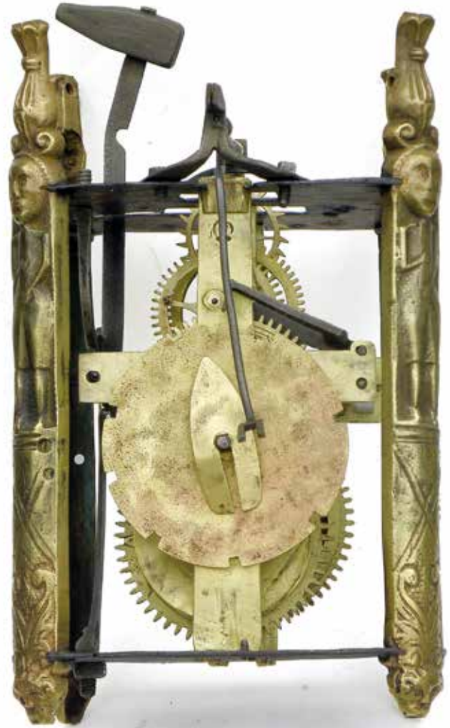
Figure 14. Rear view with the later iron back cock and crutch after conversion to anchor escapement.
