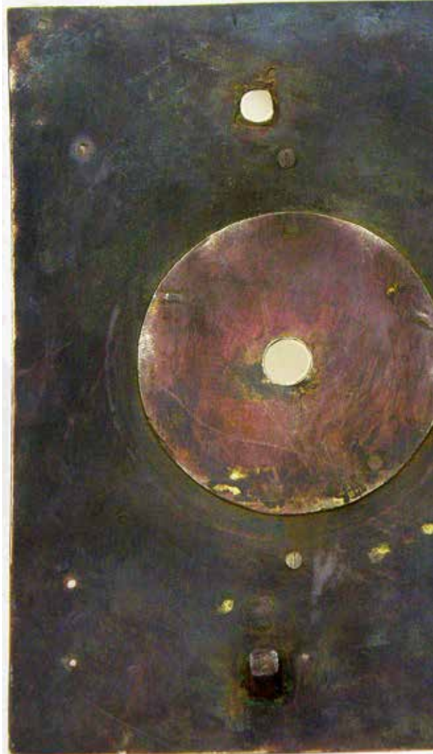
Figure 6. Rear of the dial with the insertion of a thicker central section.
