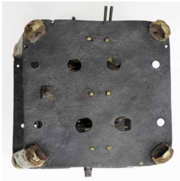
Figure 12. The iron bottom plate with two extra holes at each side where the ends of the two ropes were attached to double the duration by using pulleys for the weights and counterweights.
