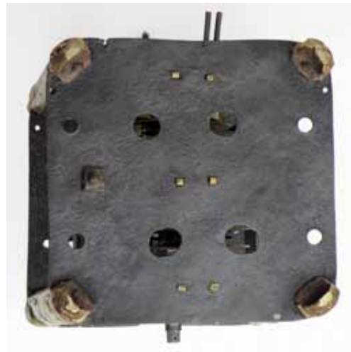
Fig. 12. The iron bottom plate with two extra holes at each side where both ends of the two ropes were attached to double the duration by using pulleys for the weights and also the counterweights.
