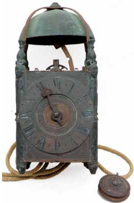
Fig. 1. Front view of the clock as found and before cleaning. The very wide chapter ring is made from modern rolled brass sheet, and the hand is made from mild steel sheet.
