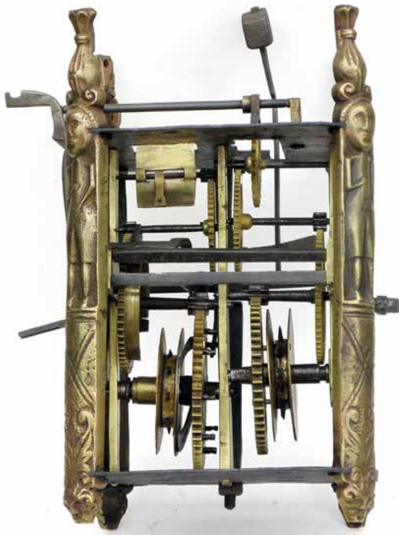
Figure 16. Movement from the left. The winding click on the going great wheel was removed during conversion to Huygens loop.
