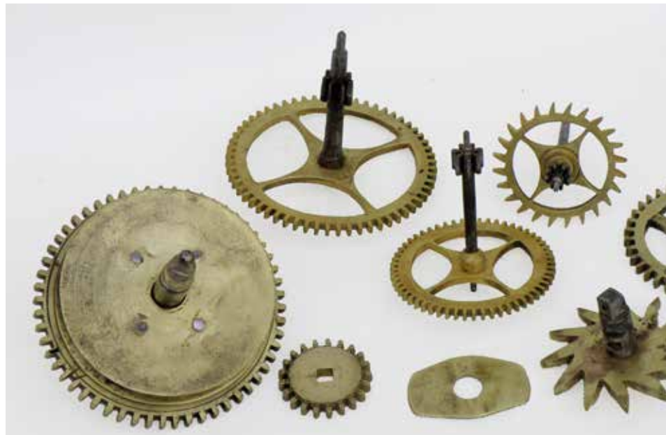
Figure 10. The four wheels of the going train after conversion to long pendulum and anchor escapement, together with the starwheel and later pinion-of-report and hour wheel.
