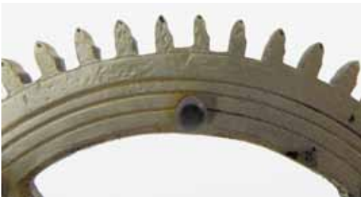
Fig. 8. Teeth of the pin wheel, have considerable wear. The punch marks on the tips show that the teeth were marked out with a dividing plate before being cut and rounded by hand.
