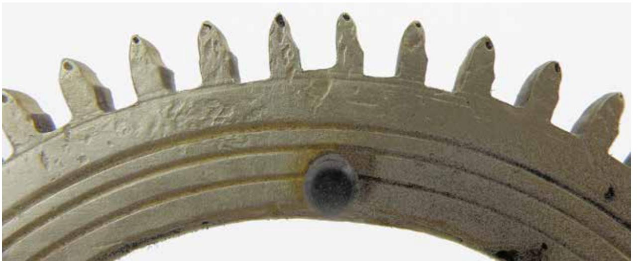
Figure 8. Teeth of the striking great wheel show considerable wear, and punch marks indicating they were cut and rounded by hand.
